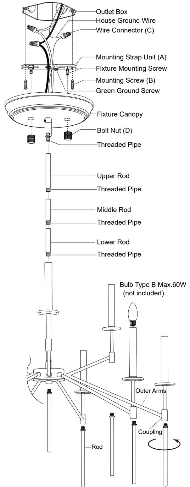
6. Attach the fixture canopy to the mounting strap unit (A) by inserting the fixture mounting screws, then secure it with two bolt nuts (D).
